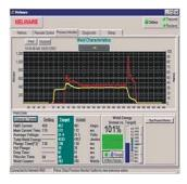
Process Monitor measures and records all critical weld inputs of each weld made
