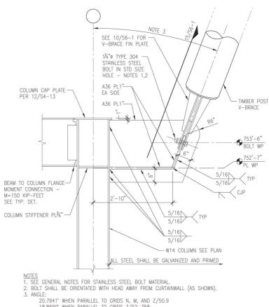
20.7941\* WHEN PARALLEL TO GRIDS N, M, AND Z/50.9 18.8690\* WHEN PARALLEL TO GRIDS Z/52-Z58 4. STRIKE THREADS ON BOLT PAST NUT.
